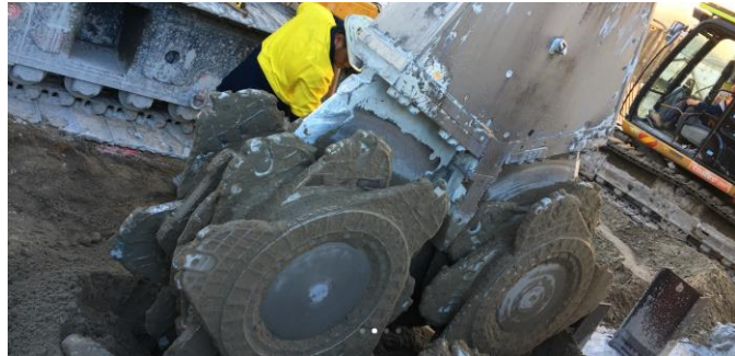
Typical Cutter Soil Mix Wall Machine
